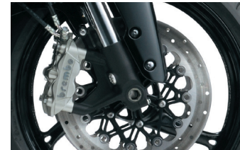
Front brake system with Brembo
