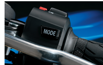
Suzuki Drive Mode Selector (S-DMS)
